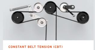
The self-adjusting belt tension technology in CBT keeps belt tension constant, which maximises belt life, minimises wear and maintains a consistent, quality cut.
