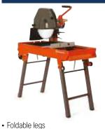
The TS 400 F is an efficient universal masonry saw with high cutting capacity for all kinds of bricks and building blocks. You can easily plunge or bevel cut at 45 degrees for maximum versatility. The robust single-piece frame with integrated conveyor rails gives great rigidity and provides longer product life.
