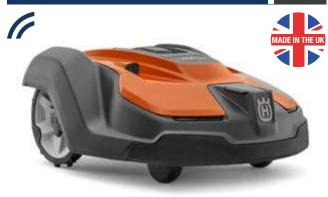
Professional robotic mower featuring Husqvarna EPOS guidance with precision area management and transport paths. With virtual boundaries you can define several work areas with different settings as well as set temporary stay-out zones. Requires EPOS reference station
