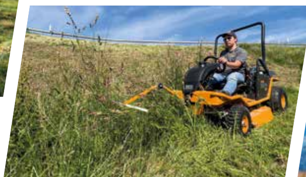
Insect-friendly Mowing with insect scare device
